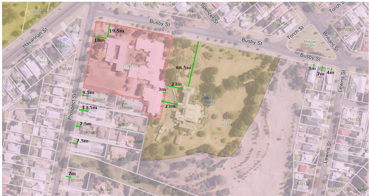
Figure 15 – Diagram of setbacks of site and surrounding buildings on the same side of the street (Busby and Prospect Streets)
